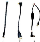
Camera and Vision Computer Cables to Bottom Gimbal End
